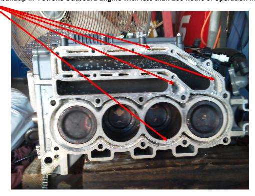
Cracked cylinder wall due to overheating from marine scale in the cooling system.
